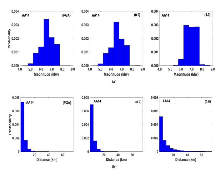
Figure A1— Disaggregation of hazard on rock, at 5,000 years return period, at the Euroseistest site for three spectral periods (PGA, 0.2s and 1.0s) (a) Disaggregation in magnitude; (b) disaggregation in hypocentral distance.
